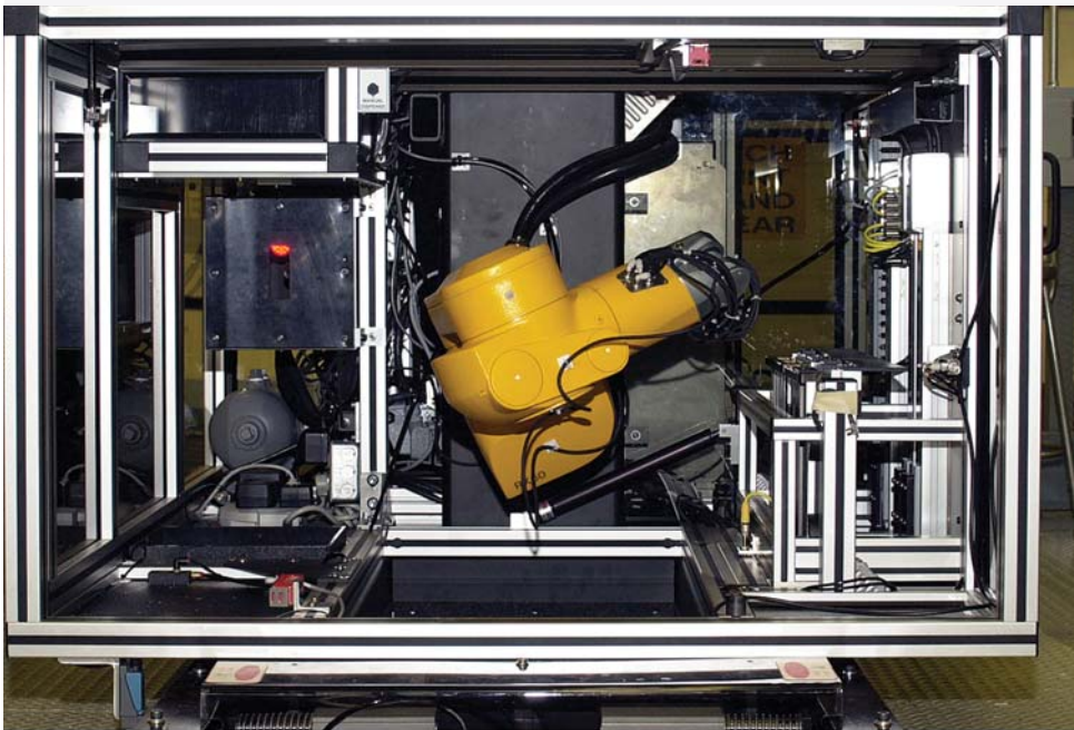
Because of the 12-by-12-foot size of the array face, this vision-guided six-axis Staubli robot is mounted on a moving so it can travel around the array face.
