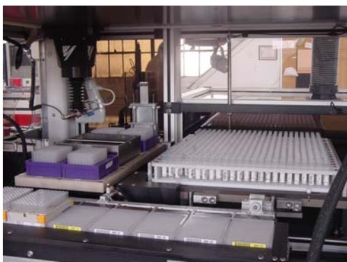
Source Tubes and Plates in Robot Work Envelope
